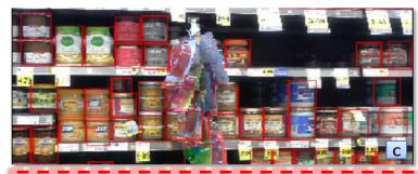
Detection in packed domains. A typical image in SKU-110K, (a) Detection results for the RetinaNet, it returns a lot of overlapping or incorrect boxes. (b) The famous two-stage detector Faster R-CNN detects few objects. (c) Our approach does precise detection.
