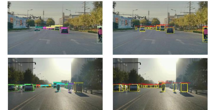
Fig. 5 The detection results of the original model and YOLOv3-2nd-block-pruning-2nd-channel-pruning model on the embedded device
