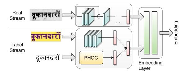
End2End network [3] for learning both textual and image embedding using a multitask loss function.
