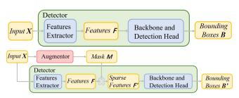
PointDrop employs an augmentation network (augmentor) to provide sparse samples and optimizes the augmentor and the detector in an adversarial way.
