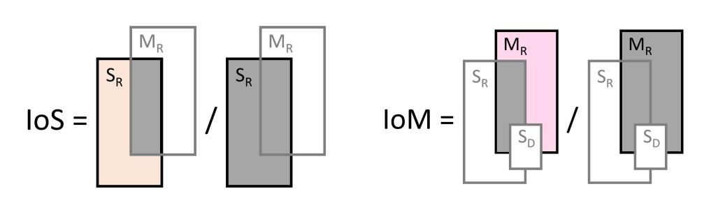
$S_R := \text{Road in segmentation}$  $S_D :=$  Dynamic objects in segmentation (e.g. car)  $M_R := \text{Road in map}$ TP := Road in segmentation and map FP := Road in segmentation, but not inmap FN := Road not in segmentation, but in map
