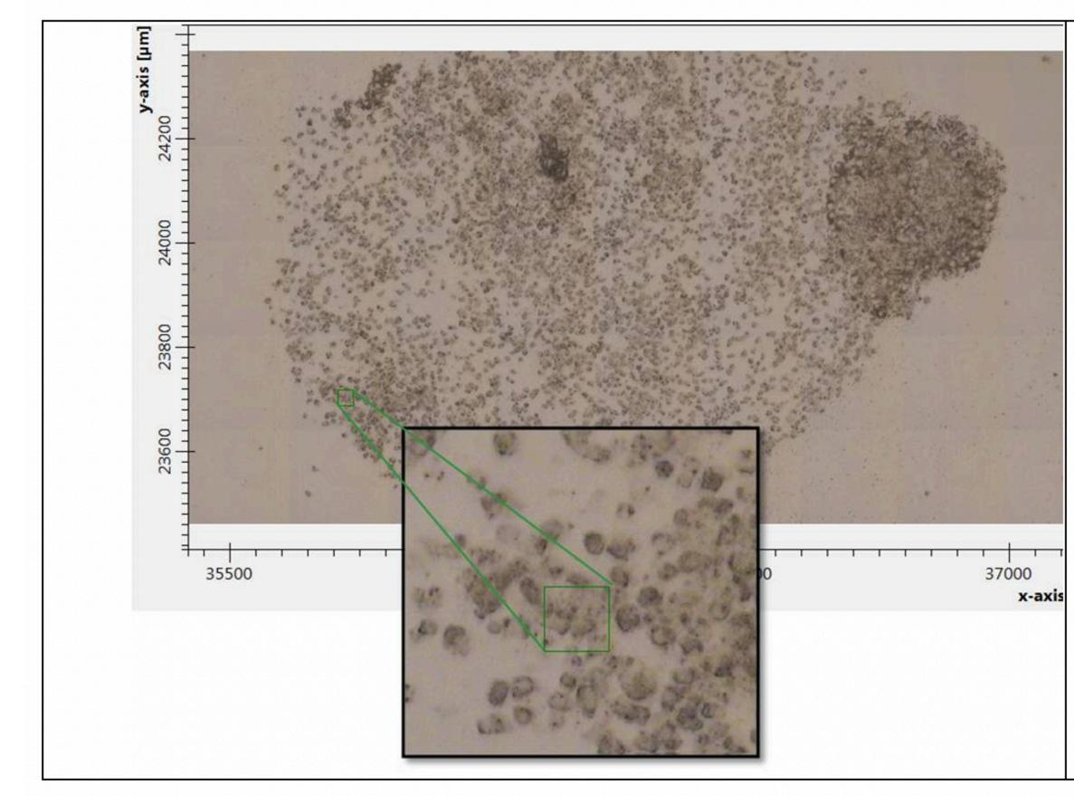
Microphotograph of a living GC sample inside the microfluidic device. The green square represents a selected area (30x30 µm) on which the IR acquisition was performed.
