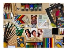
Computation method : Modulation transfer function (Relation between content photographed and resulting image) and Acutance (Sharpness measure derived from the MTF)
