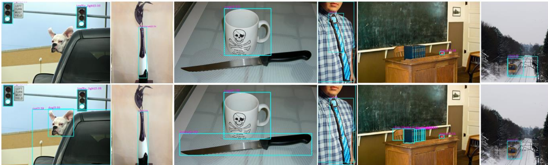
Fig. 6. Some comparison examples between FCOS (top) and our detector with BMFPN (bottom). Both are using ResNet-50 as backbone. Our BMFPN helps finding more challenging objects.
